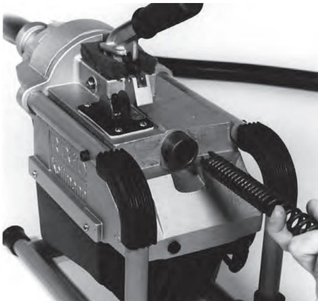
Figure 5 – Inserting Cable Into Front Of Machine
