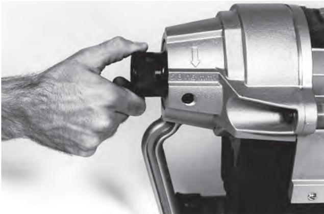
Figure 10 – Jaw Set Adjustment
