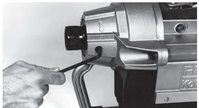
**Figure 9 – Loosen the Set Screw**
