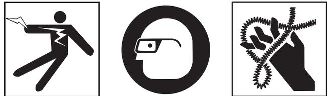
**Do not place machine in water. Water entering the motor can result in electrical shock.**
